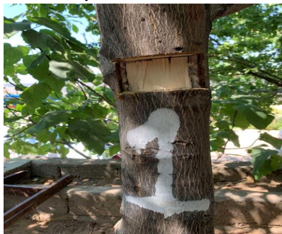
Figure (1) The method of taking wood sample from the tree at (d.b.h.).
