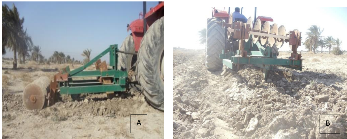
Figure (1) picture of the machine (A) with discs and (B) without the discs
