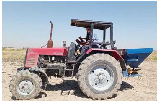
Figure.2- A mounted type seed spreader connected to the power take off shaft at rear of Belarus 820tractor
